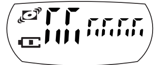
test pattern 2 (alternate segments activated)
